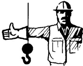
**RAISE BOOM** - Arm extended, fingers closed, thumb pointed upwards.
