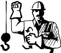
**TRAVEL** - (one tracks) Lock the track on side indicated by raised fist. Travel opposite track in direction indicated by circular motion of other fist, rotated vertically in front of the body (for crawler cranes only).
