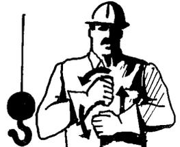
**TRAVEL** - (both tracks) Use both fists in front of body, making a circular motion about each other, indicating direction of travel.
