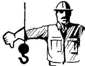
**LOWER BOOM** - Arm extended, fingers closed, thumb pointed downward.
